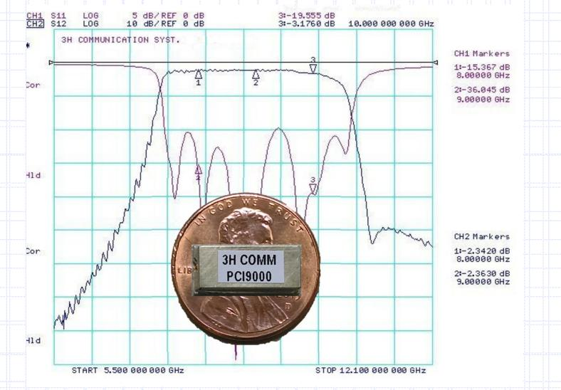
This X-Band, Miniature, LEADLESS, SMT, Pico filter offers low passband insertion loss of <3.5 dB with a VSWR 2.0:1. The filter size is **0.43"L x 0.28"W x 0.15 "H**. The filter is manufactured for automated assembly processes and is designed to meet Mil-Std-202 conditions.
